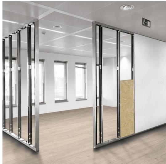
Figure 44 – Impression of a traditional metal stud wand and the Juunoo wall system
