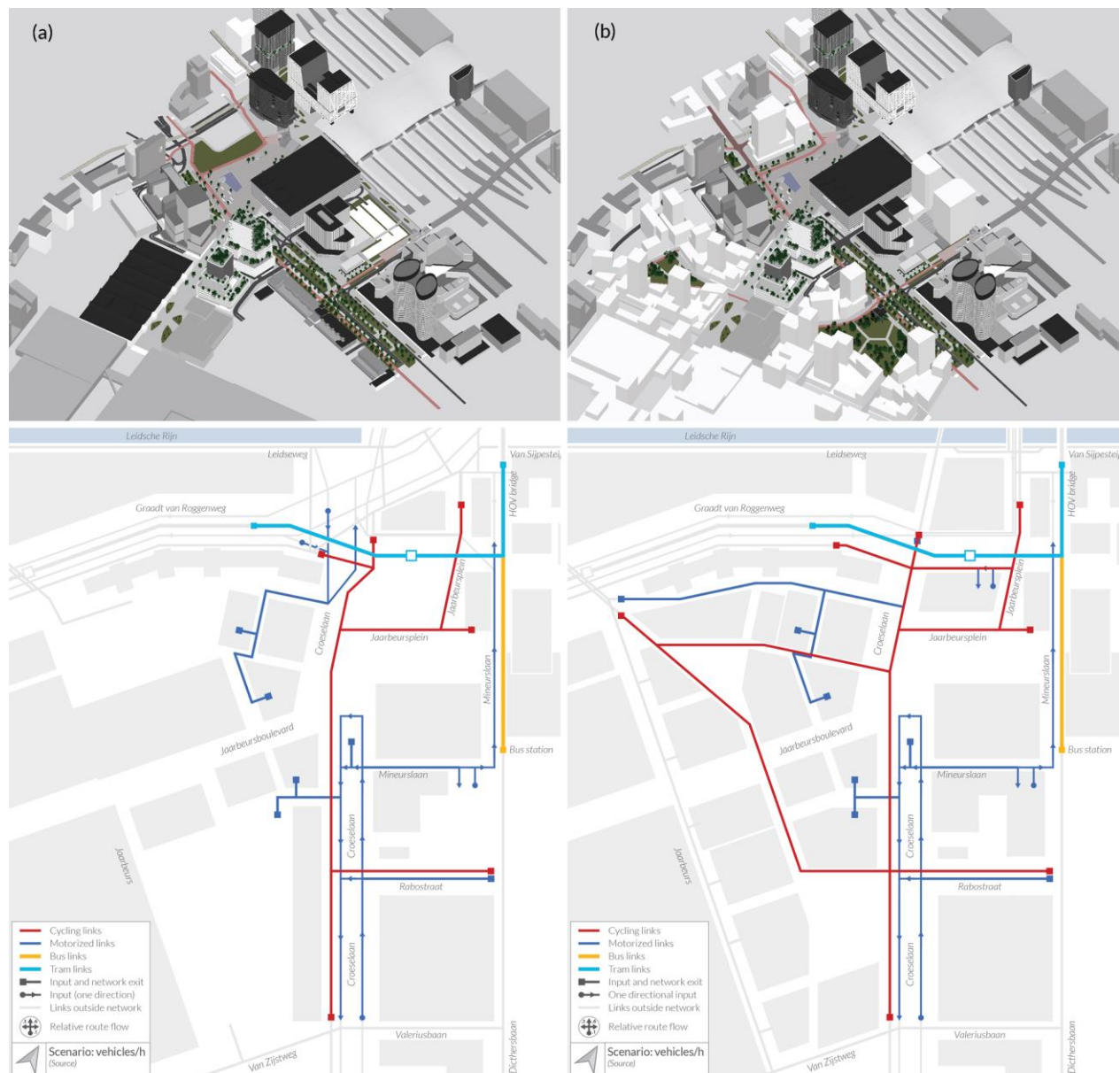
Figure 4.7: 3D model and schematic overview of network and of: a) base and b) future network
