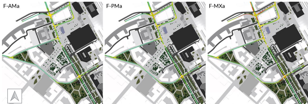
Figure 4.19: Average speed during simulations in future network
