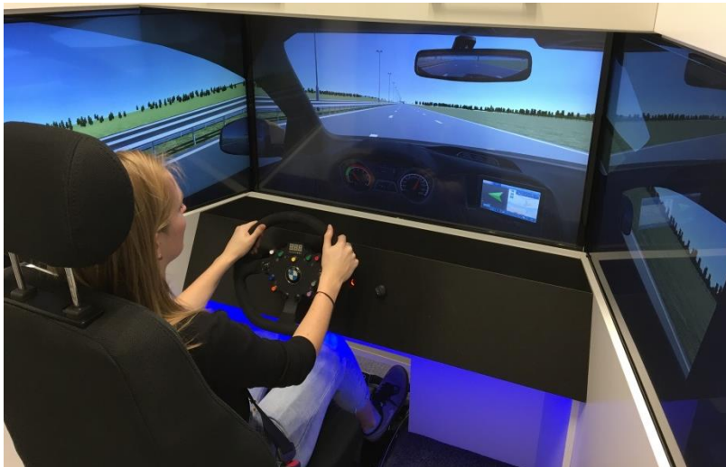
Figure 5-1. Driving simulator hardware
