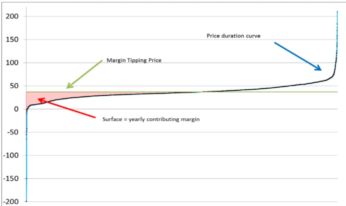
Figure 12: The price-duration curve of the electricity spot market price including the margin tipping point in €/MW for west Denmark for the year 2012; source: (Stikkelman & Lans, 2014)
