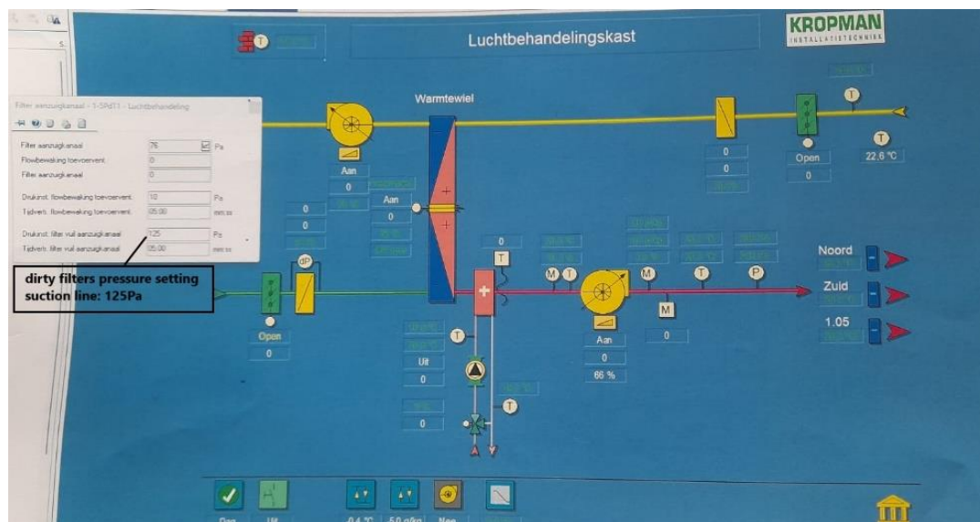
Figure 32: Screenshot from AHU BMS
