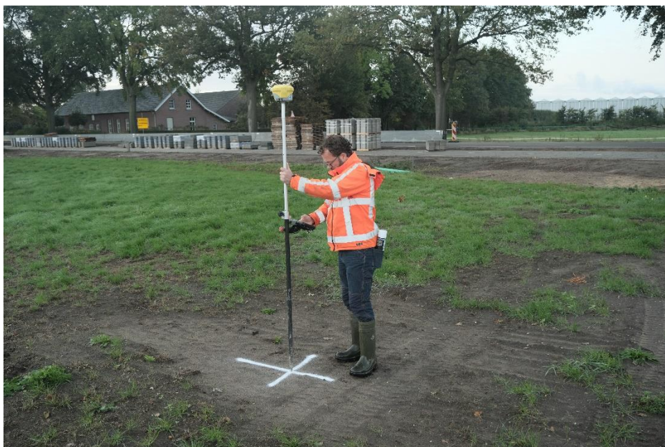
Figure 19. Task 006 in practise; setting GCPs and determining its position.
