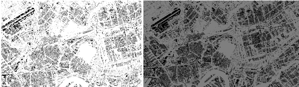
Figure 67. Flood inundation layers [TIF] representing a rainfall intensity of 70mm per 2 hours (left) and of 140mm per 2 hours (right).
