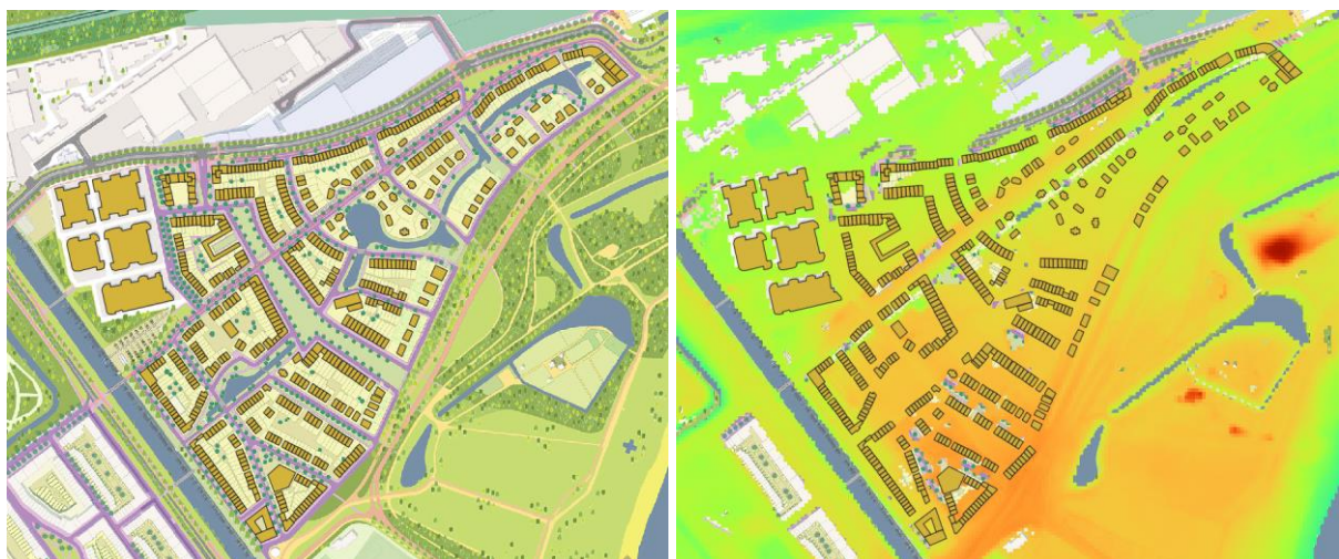
Figures 96 and 97. Shapefile of Nieuw Kralingen (left) including the AHN of the area, where the increasing height of the surface area is indicated by the intensity of red (right).
