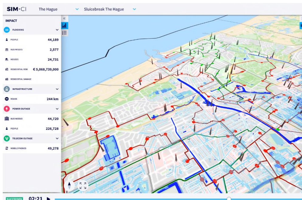
Figure 7. User interface of the SIM-CI software platform (NGInfra, n.d.).
