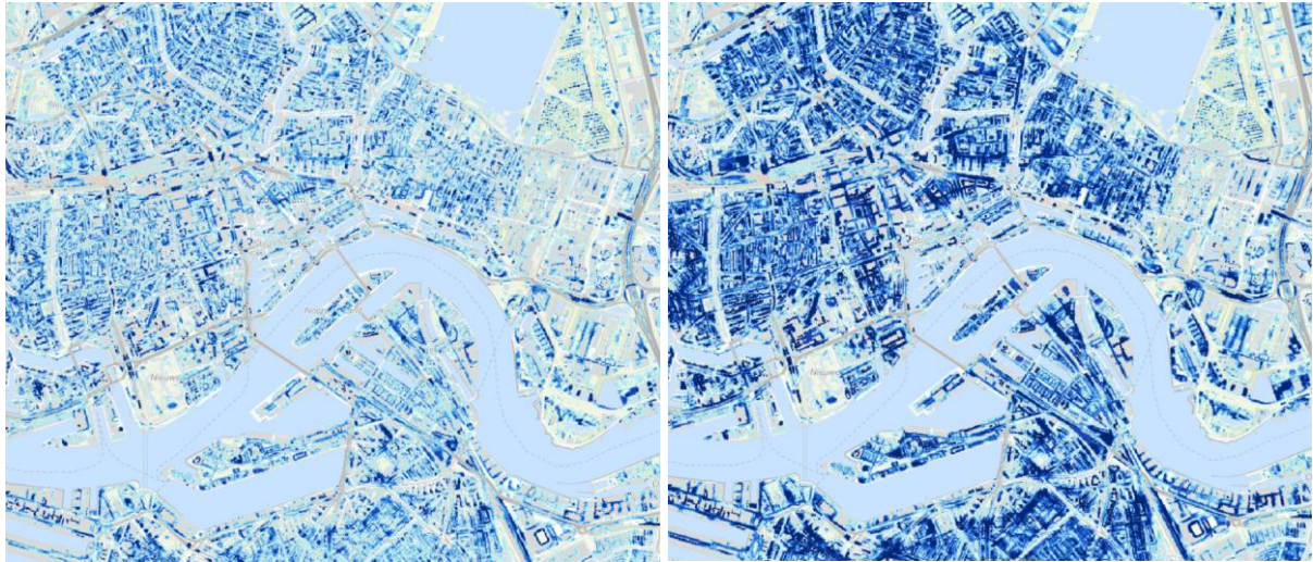
Figures 31 & 32. Flood inundation map of Rotterdam resulting from a rainfall intensity of 70 millimetres (left) and 140 millimetres (right) per 2 hours (Klimaateffectatlas, n.d.).
