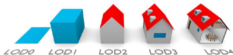
Figure 17. The five official LODs of a building in CityGML 2.0 (Open Geospatial Consortium, 2012).
